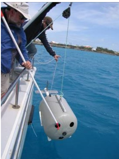
Fig. 10. Research technicians lowering the drop-camera array into the water. During filming, a separate video cable was also connected to the drop camera array separately.
