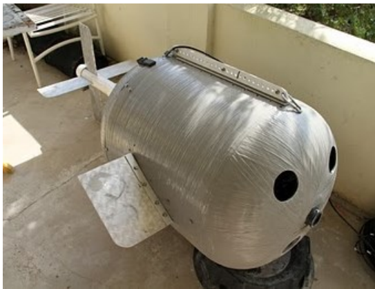
Fig. 9. A front-view of the camera housing. The two upper holes will allow two forward-facing circular HD video cameras to film fish assemblages as the array moved through the water over the reef. The lower circular hole is for the analogue video camera, which provides a live video feed to the researchers so that the camera array can be raised and lowered by rope to avoid objects while underway.
