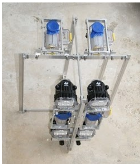
Fig. 7. Four underwater camera housings (blue) and 4 underwater lights (black), mounted on the aluminium frame which will be inserted into the drop-camera housing. An analogue camera was also mounted onto this same frame below the uppermost video housings.
