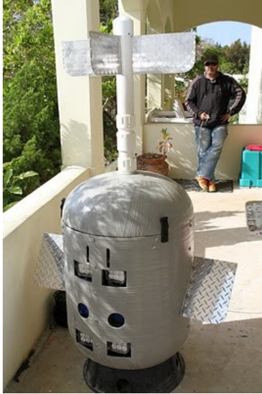
Fig. 8. A ventral-side photograph of the completed drop-camera array housing, constructed from a fiberglass water pressure tank. The 4 rectangular UW lights and two circular downward-facing HD video camera ports can be seen. The housing is sitting in a stand, and a pvc pipe supports a tail-fin. Side fins were added to reduce yaw. Weights were later added to the underside to further stabilize the array.
